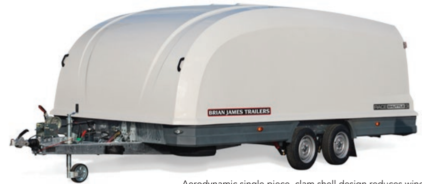
Aerodynamic single piece, clam shell design reduces wind drag and improves towing fuel consumption.
